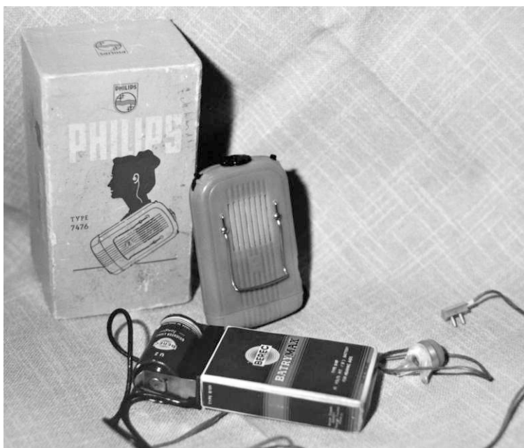
Ill. 11: Small design with subminiature tubes
